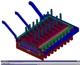
Have developed the software Dyna/Marc that simulates the dynamic behaviour of an aluminum reduction cell. Dyna/Marc is commercialised by GéniSim Inc.
