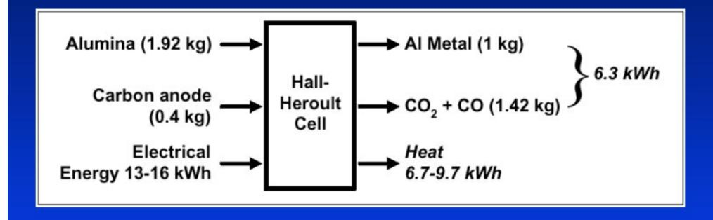
Over long periods of time neither mass or energy can accumulate in a cell, it must globally operates in mass and thermal balance
