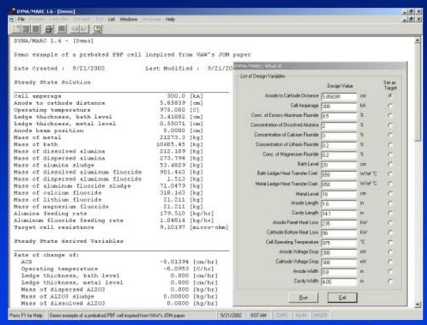
Steady/MARC, lump parameters+: simplest and fastest approach
