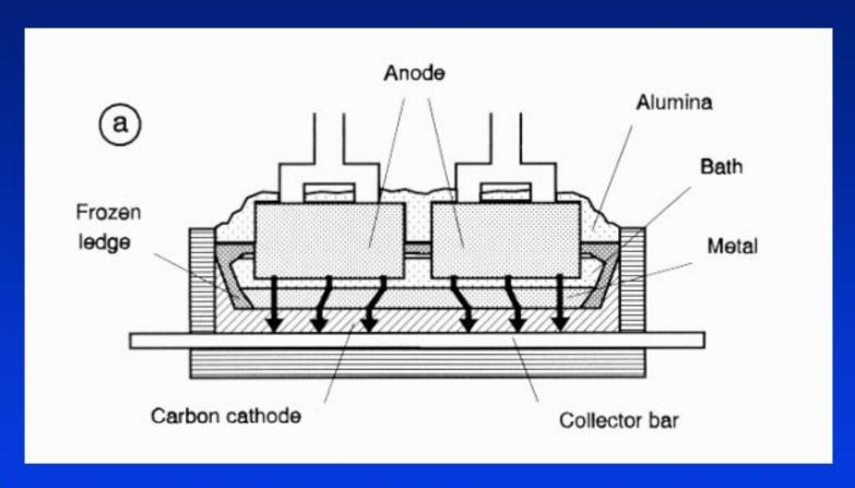
To ensure that the cell is operating with the optimum ledge protection
