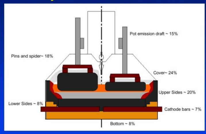
Heat Partition depends on the anode and cathode lining design
