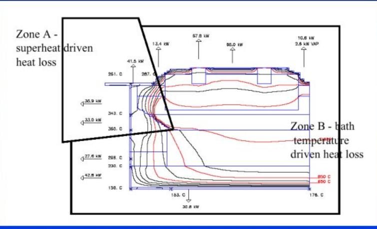
The cell superheat dictates the amount of heat dissipates in zone A
