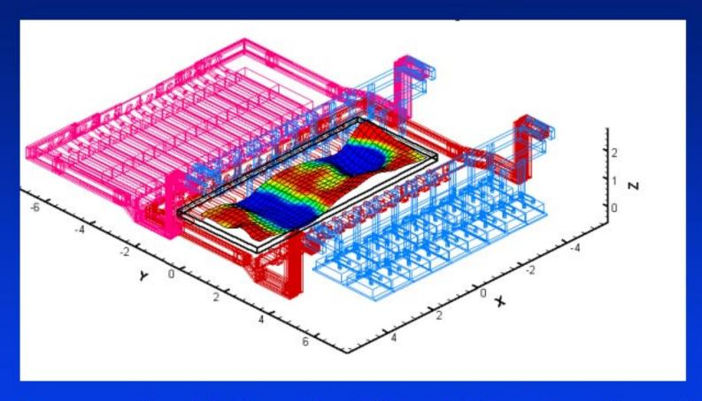
To ensure the stability of the bath-metal interface of the cell
