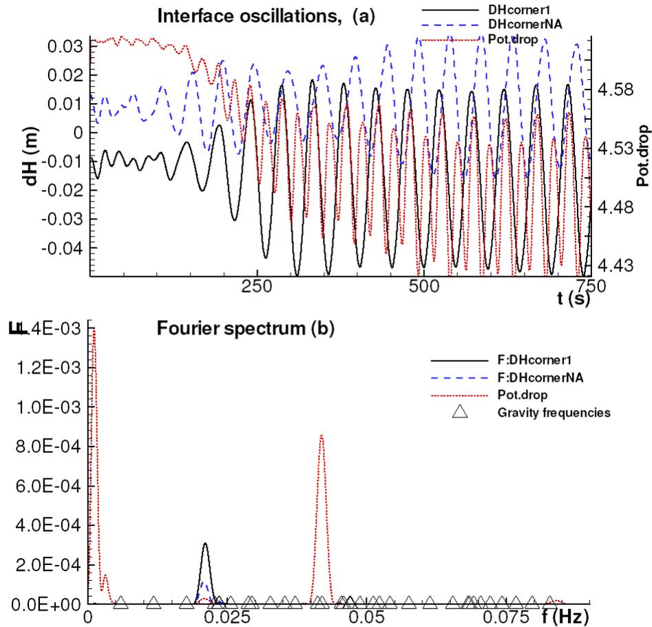
Figure 16: MHD-Valdis model liquid metal pad and cell voltage oscillation
