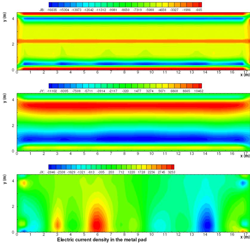
Figure 12: MHD-Valdis model metal pad current density field solution
