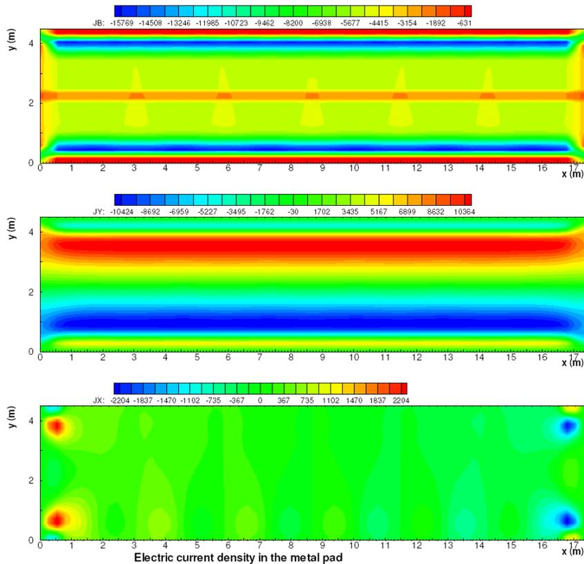
Figure 20: MHD-Valdis model metal pad current density field solution
