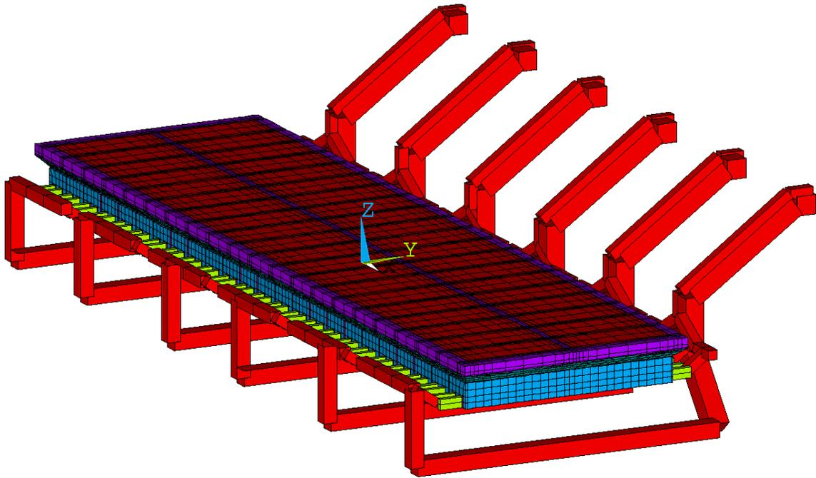
Figure 3: Full cell partially 1D ANSYS® based model mesh
