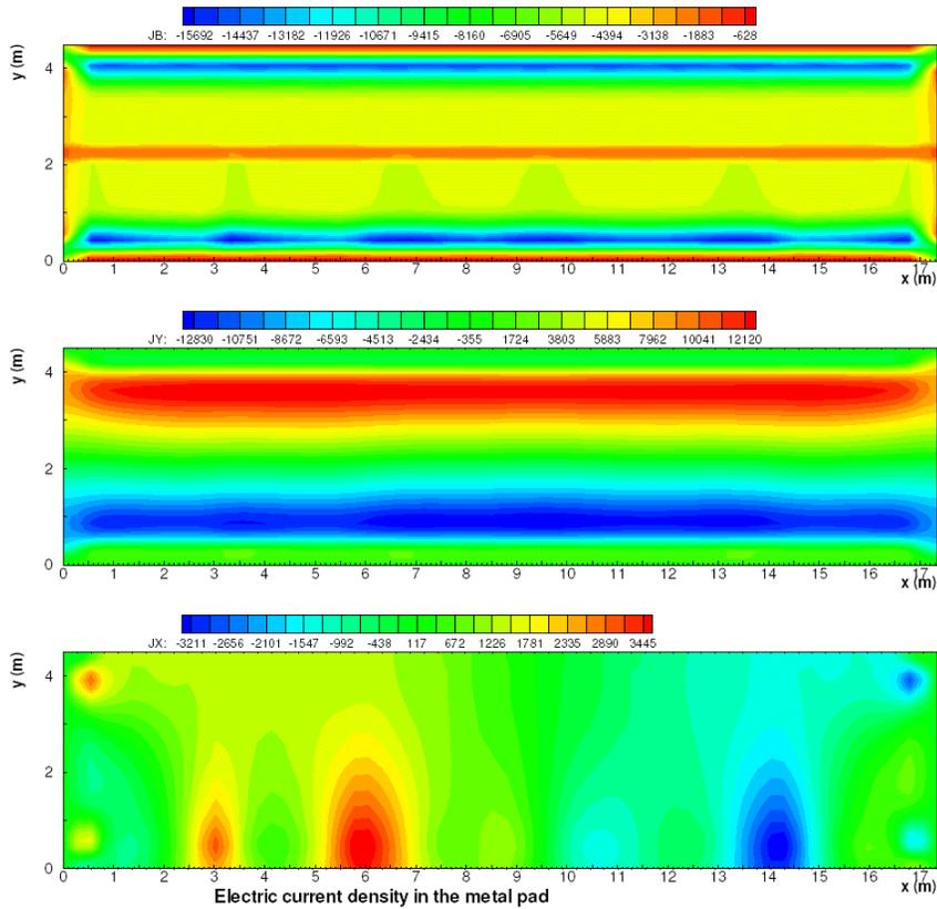
Figure 6: MHD-Valdis model metal pad current density field solution:  $J_z$  at bottom,  $J_y$  and  $J_x$  depth average.
