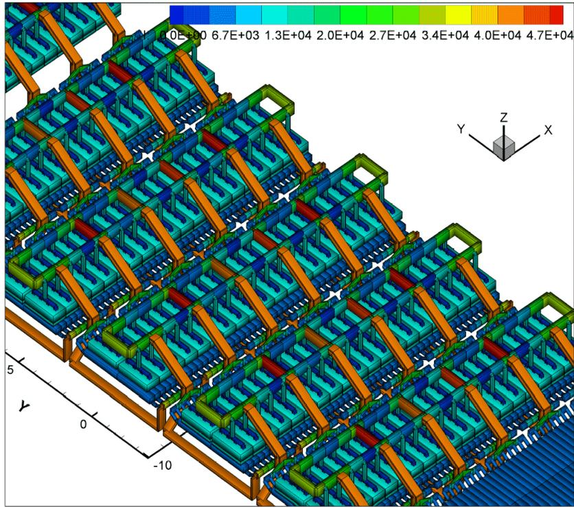
Figure 5: MHD-Valdis electric network model mesh
