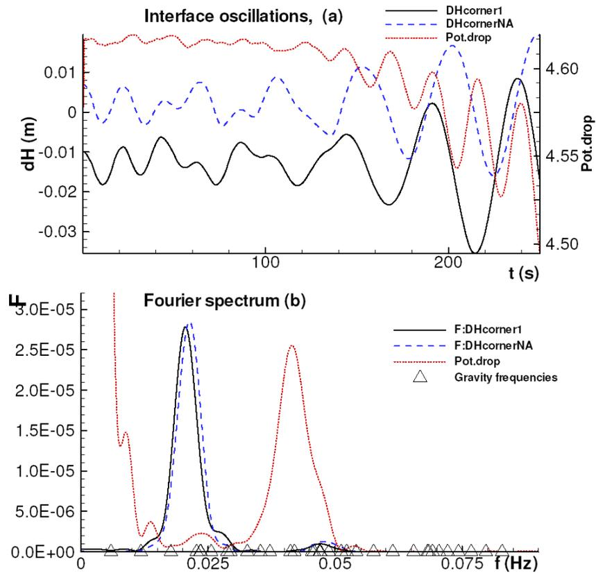
Figure 23: MHD-Valdis model liquid metal pad and cell voltage oscillation
