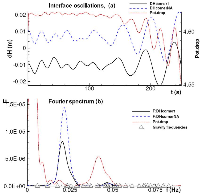
Figure 21: MHD-Valdis model liquid metal pad and cell voltage oscillation
