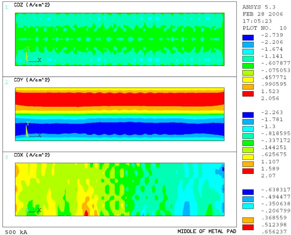
Figure 8: Full cell partial 1D model metal pad current density field solution
