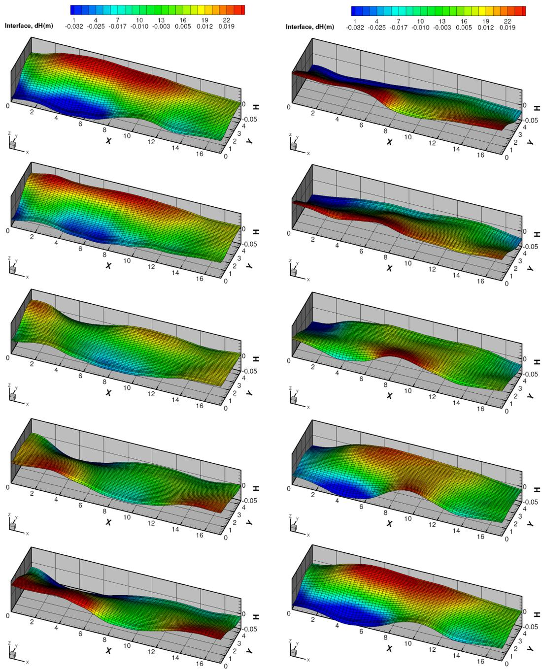
Figure 17: MHD-Valdis model bath-metal interface wave pattern
