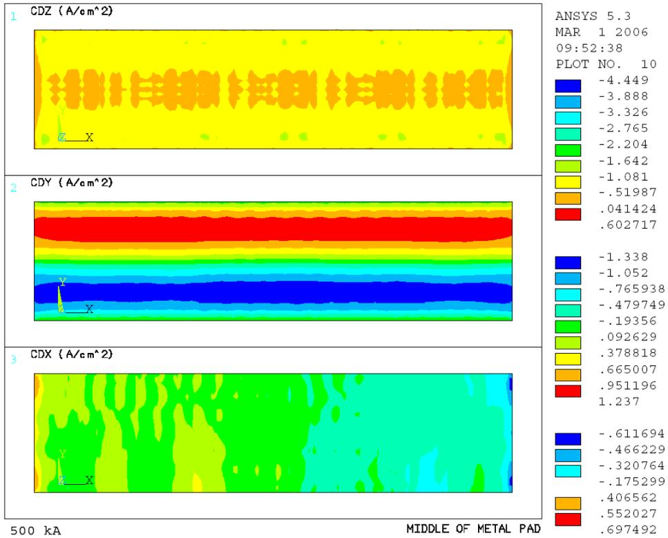
Figure 11: Full cell partial 1D model metal pad current density field solution
