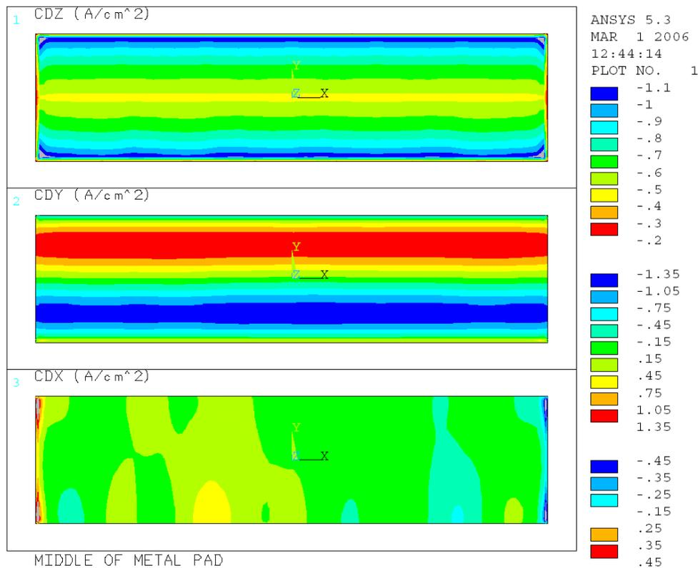
Figure 10: Full cell 3D model metal pad current density field solution
