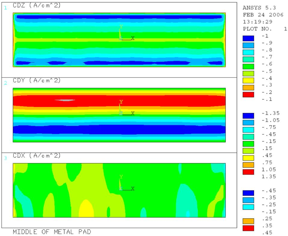
Figure 2: Full cell 3D model metal pad current density field solution
