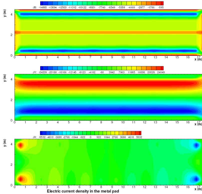
Figure 18: MHD-Valdis model metal pad current density field solution
