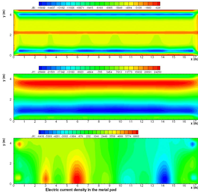
Figure 9: MHD-Valdis model metal pad current density field solution
