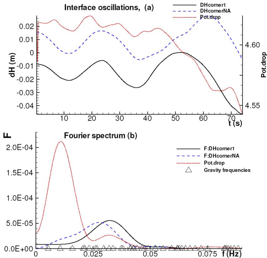
Figure 19: MHD-Valdis model liquid metal pad and cell voltage oscillation
