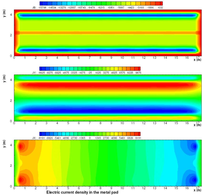
Figure 22: MHD-Valdis model metal pad current density field solution
