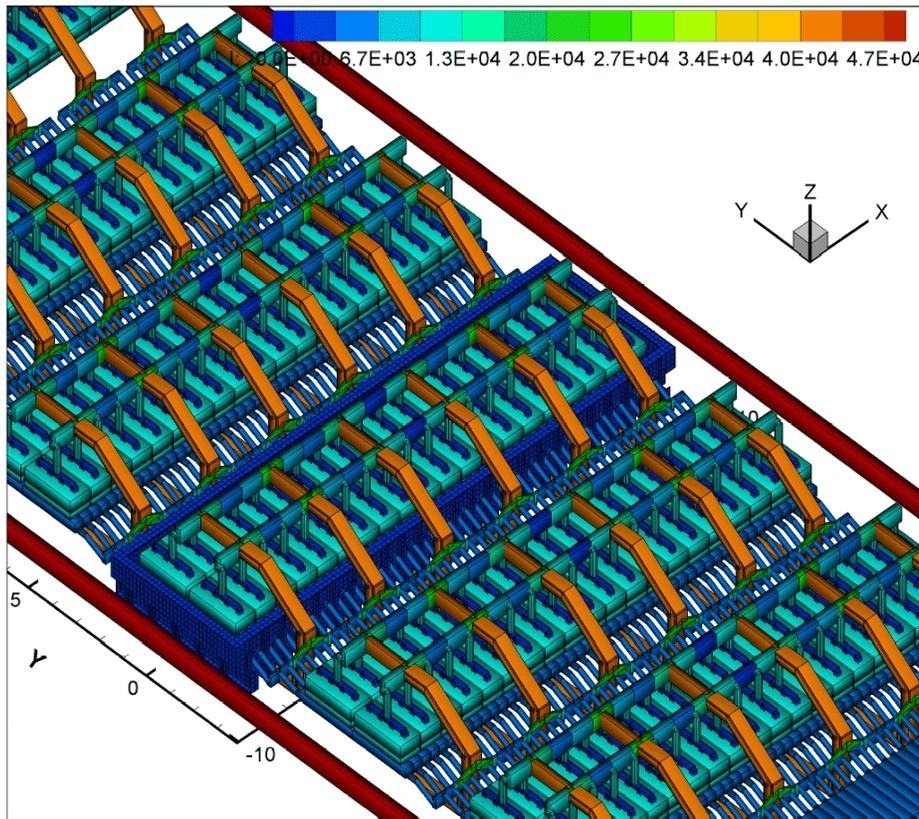
Figure 13: MHD-Valdis electric network model mesh with compensation loop
