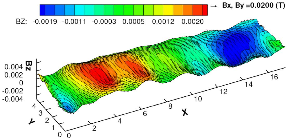
Figure 15: MHD-Valdis model metal pad magnetic field solution
