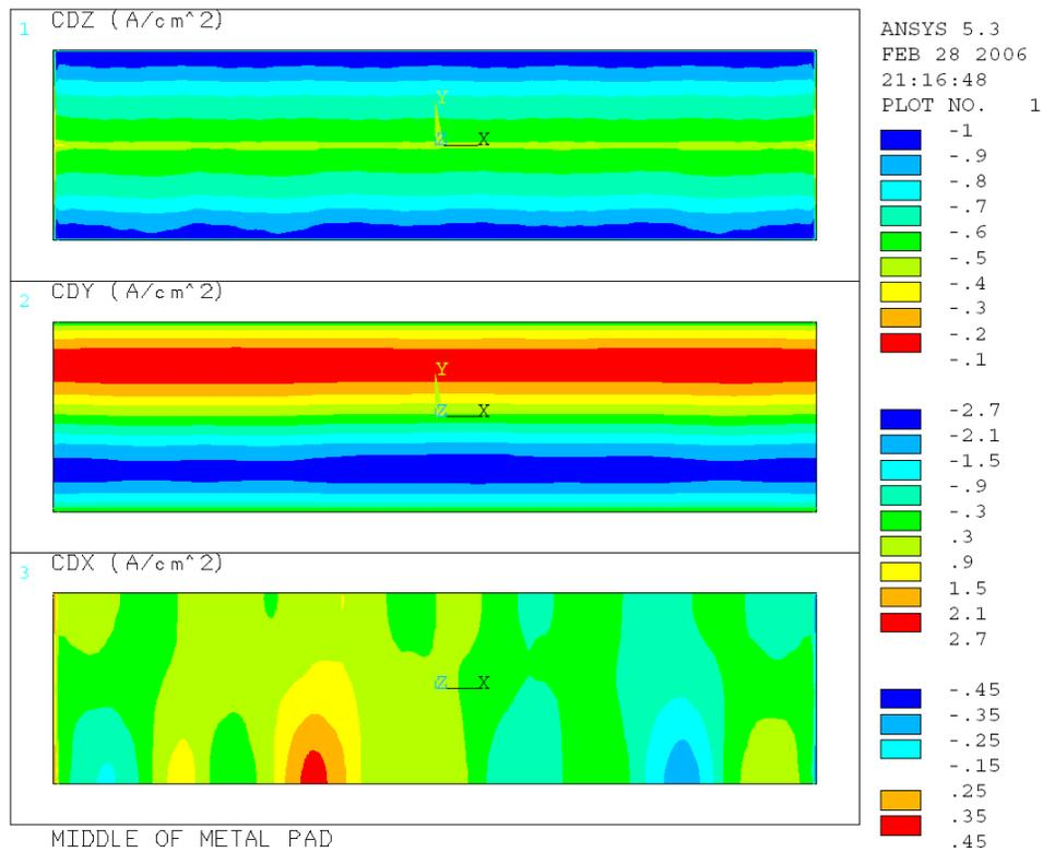
Figure 7: Full cell 3D model metal pad current density field solution
