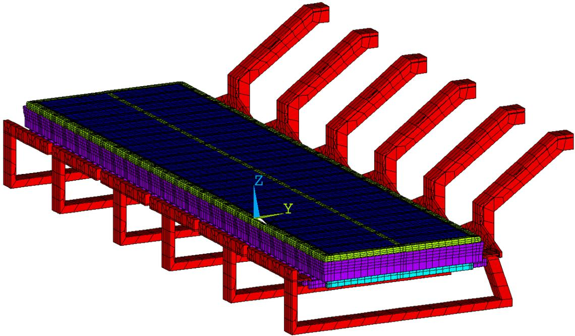
Figure 1: Full cell 3D ANSYS® based model mesh
