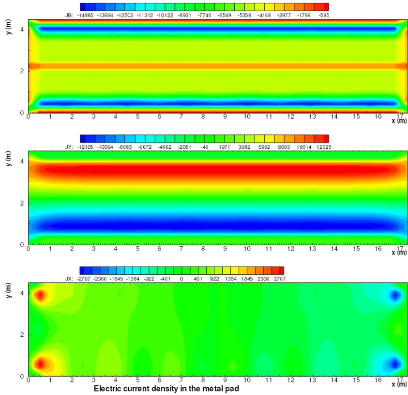
Figure 14: MHD-Valdis model metal pad current density field solution
