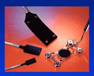
Bruggeman[1], clearly expressed the current conventional wisdom of the industry by specifying that heat flux transducer must be used to carry out cell heat loss measurement campaigns.
