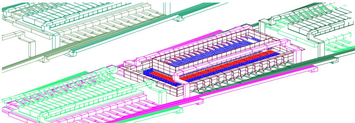
Figure 2. Soderberg horizontal stud reduction cell Autocad representation of the elements used for the magnetic field and electric current modelling.
