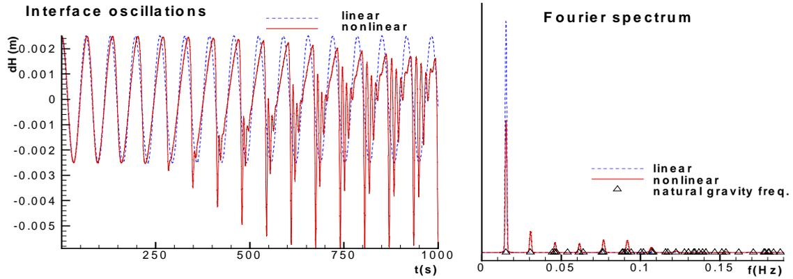
Figure 1. Linear and non-linear wave evolution from the (1,0) natural gravity wave initial perturbation.
