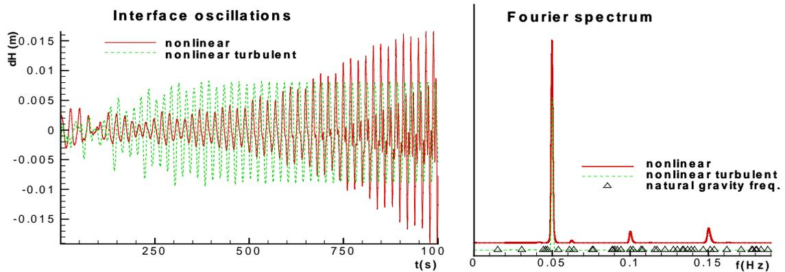
Figure 3. Non-linear wave evolution from the (1,0) perturbation with the effect from the magnetic field for the Soderberg cell.
