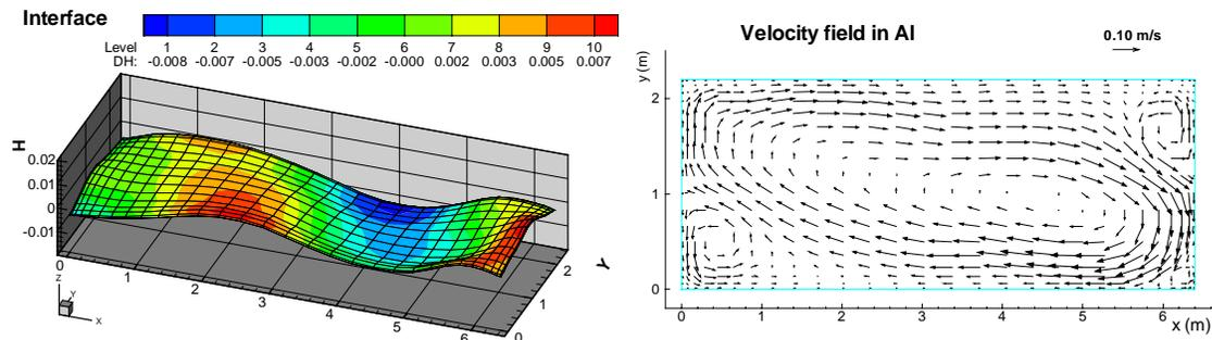
Figure 4. The instantaneous interface shape and the turbulent velocity field in the liquid metal at  $t = 1000s$ .
