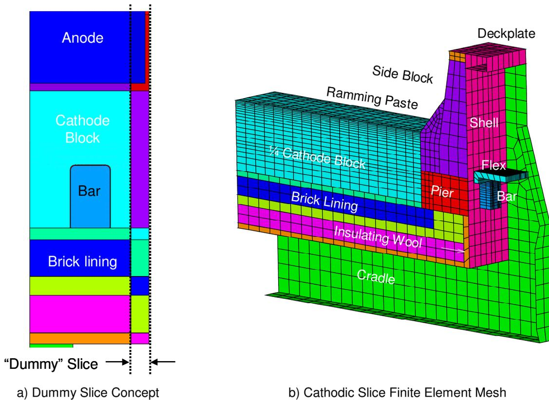
**Figure 2 Cell Slice Model Details.**
