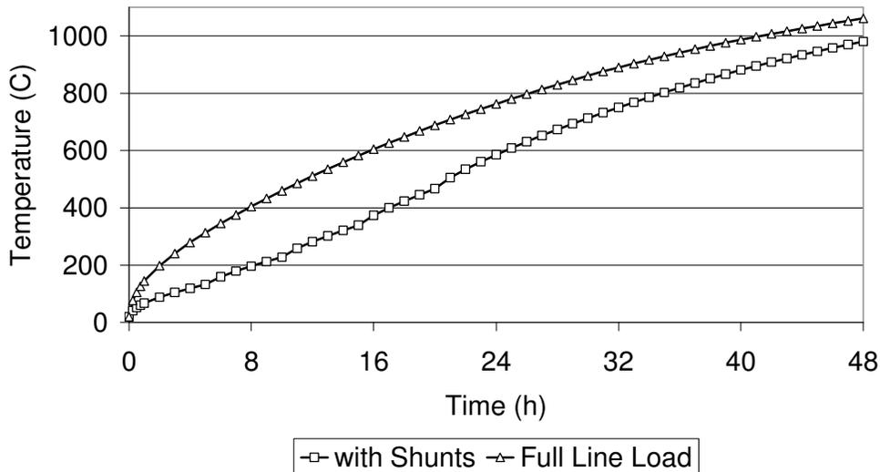
**Figure 7 Evolution of Maximum Cathode Surface Temperature.**
