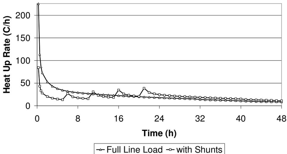
**Figure 8 Calculated Heat up Rate at Maximum Surface Temperature Location.**
