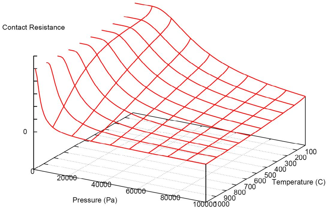
**Figure 4 Electrical Contact Resistance at the Cast Iron to Cathode Block Interface.**
