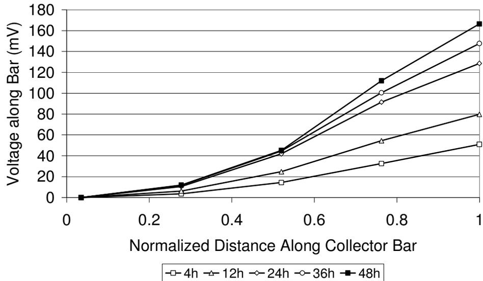
**Figure 14 Collector Bar Current Pickup for Full Line Load Preheating.**
