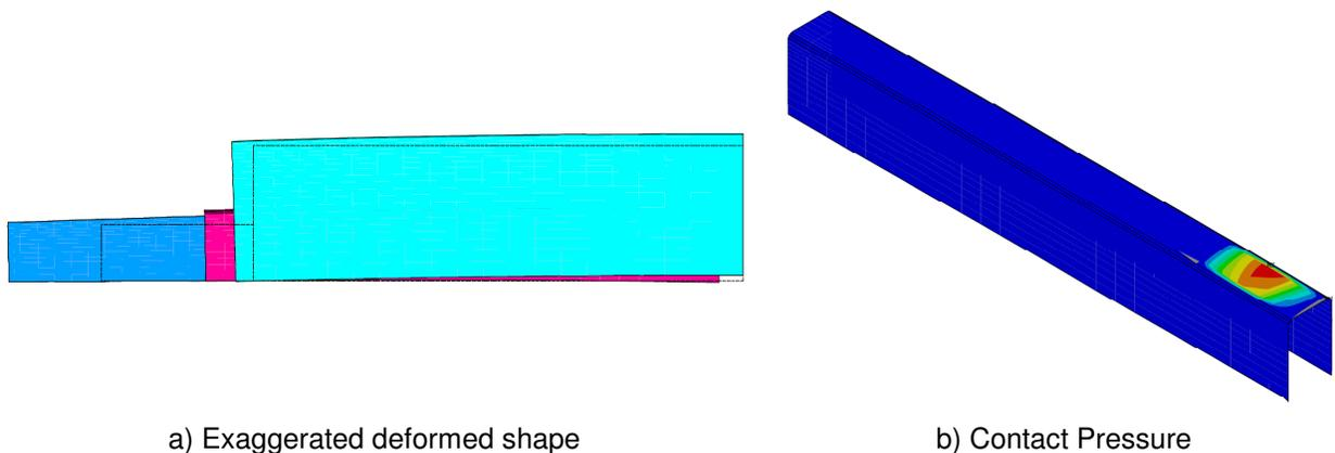
**Figure 13 Localisation of Cast Iron to Carbon Contact Zone after 48 hours, with Shunts.**
