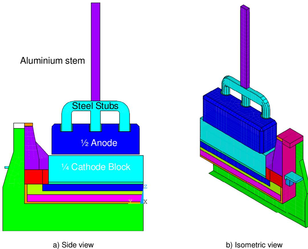
**Figure 1 Cell Slice Finite Element Geometry**
