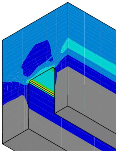
a) First Principal Permanent Tensile Strain in the Cathode Block Slot at 48h, with Shunts
