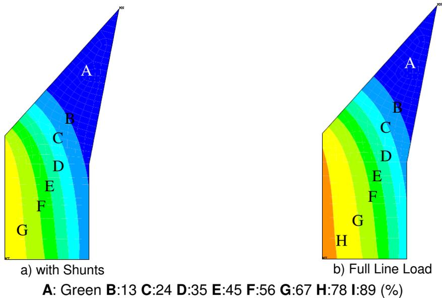
**Figure 12 Ramming paste baking index at the end of preheating**
