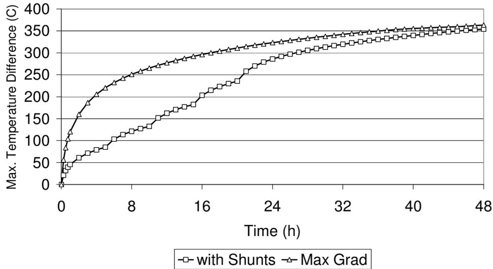
**Figure 9 Evolution of Maximum Temperature Difference in Cathode Block.**
