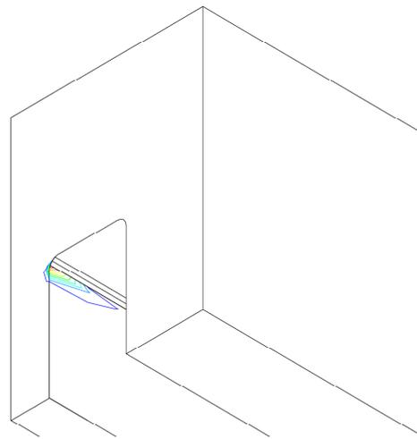
b) Softening Parameter in the Cathode Block Slot at 48 h, Full Line Load.
