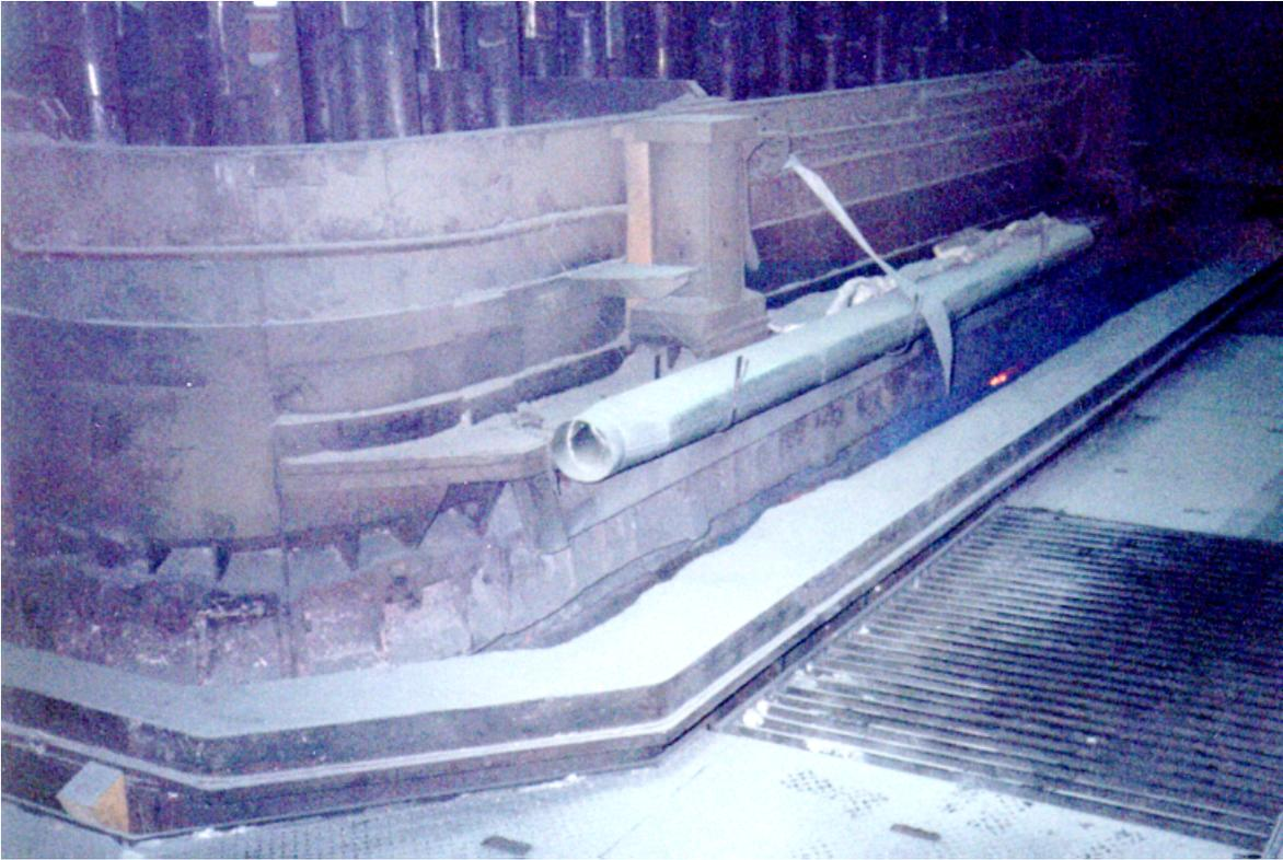
Figure 1: VS Söderberg Cell with Experimental Hood
